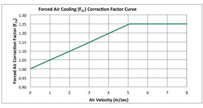
Figure 30. Forced (air) cooling correction factor (F<sub>FC</sub>) curve
