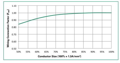
Figure 31. Wiring connection factor (F<sub>WR</sub>) curve
