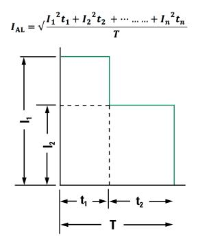
Figure 27. Varying load current (cyclic current)
